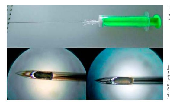
Even fine structures, like the epidural needle shown here, can be cleaned with CNP.
