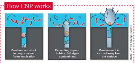
The asymmetrical volume flow creates a pump effect. When the bubbles burst, there is an exchange of media in the capillaries and drill holes which helps remove contaminants.
