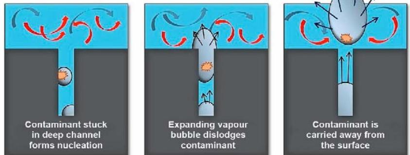
The asymmetrical volume flow creates a pump effect. When the bubbles burst, there is an exchange of media in the capillaries and drill holes which helps remove contaminants.
