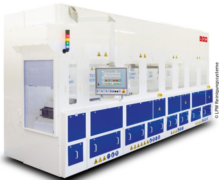
The benefits of enclosed chamber machines, in this case an automated top-loader, include the hermetically sealed cleaning chambers.
