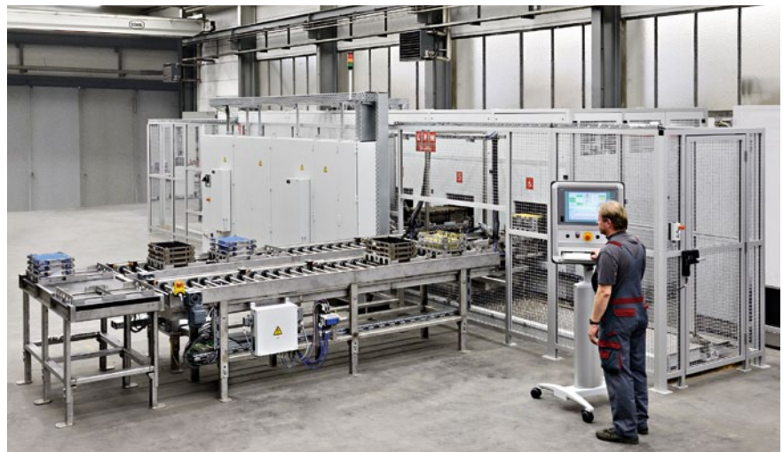
The six-chamber system provides interim and final cleaning processes for injection components and meets the highest standards of cleanliness.
